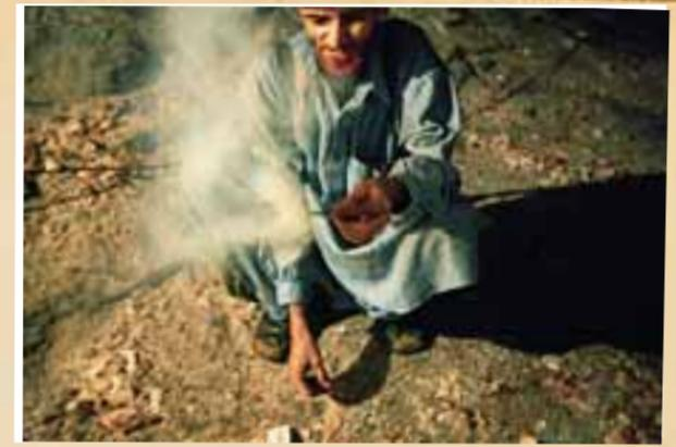
A two-meter-deep hole is drilled into the wall of salt with a hand drill and filled with gun powder from a bag; it's then exploded with a fuse. The dislodged pieces are chopped up and, after 400 million years in total darkness, carried outside.
